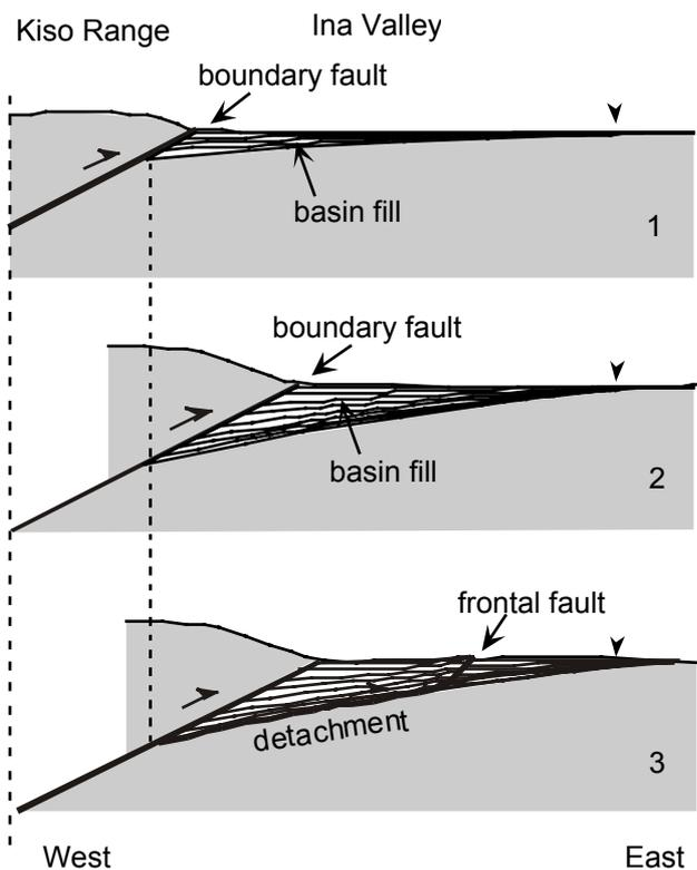
**Figure 3.** Thrust-front migration in the Ina Valley Fault Zone, central Japan (modified from Ikeda, 1983).
