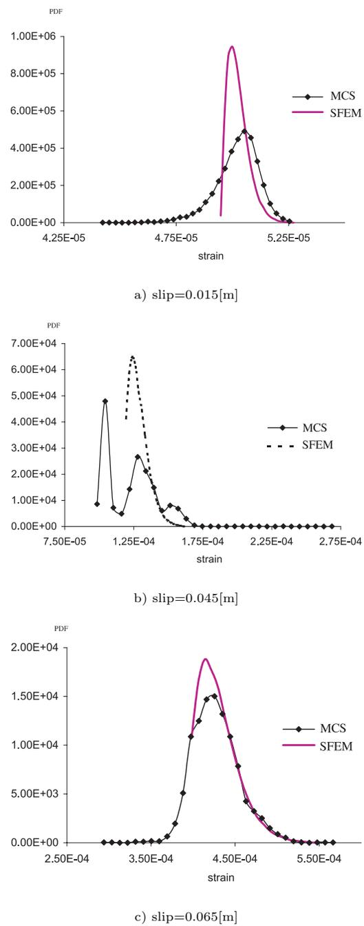
Fig. 7 Evolution of PDF of maximum shear strain.
