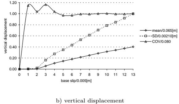
**Fig. 10** Change in mean and SD of surface displacement.
