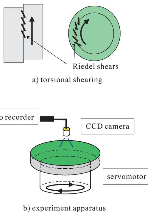
**Fig. 1** Schematic view of model experiment.
