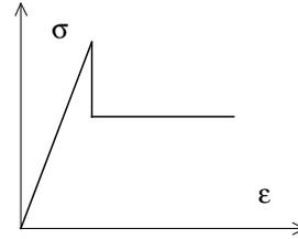
Figure 4 Assumed Stress-strain curve for a material point
