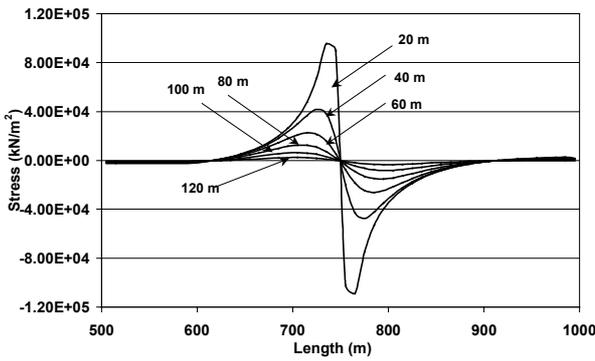
Fig. 6. Stresses in vertical direction in soil deposit at regular intervals (Case 1)
