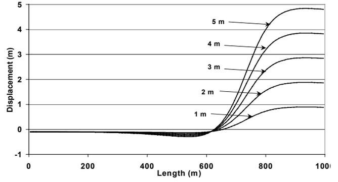
Fig. 7. Surface displacement at each 1-m displacement of hanging wall (Case 2: elastic analysis, dip angle =  $45^0$ )
