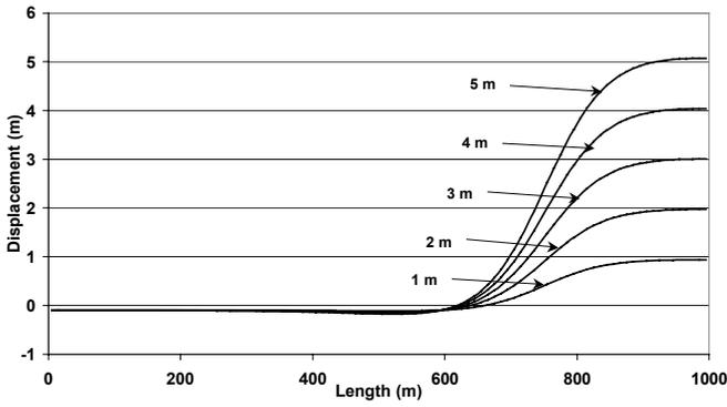
Fig. 5. Surface displacement at each 1-m displacement of hanging wall (Case 1: elastic analysis, dip angle =  $90^0$ )
