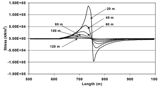
Fig. 8. Stresses in vertical direction in soil deposit at regular intervals (Case 2)
